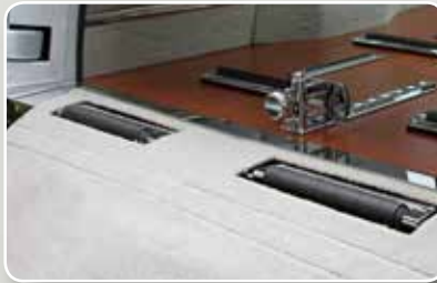
Eagle includes a short rear bumper protector and a quick-release adjustable bier pin.
